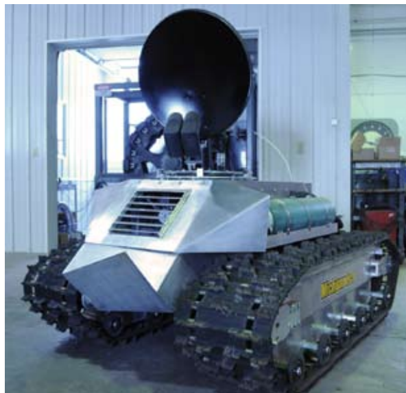
Little Brother (left) and Big Brother (right) unmanned vehicles, operated by fuels cells, are being designed, built, and tested at the Keweenaw Research Center.
